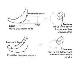
Controlled by the sensor values, two servo motors mounted at a right angle drive the camera in two axes (tilt and pan).
