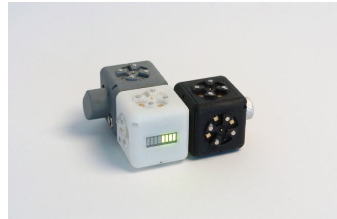
Figure 1. A simple roBlocks robot.
