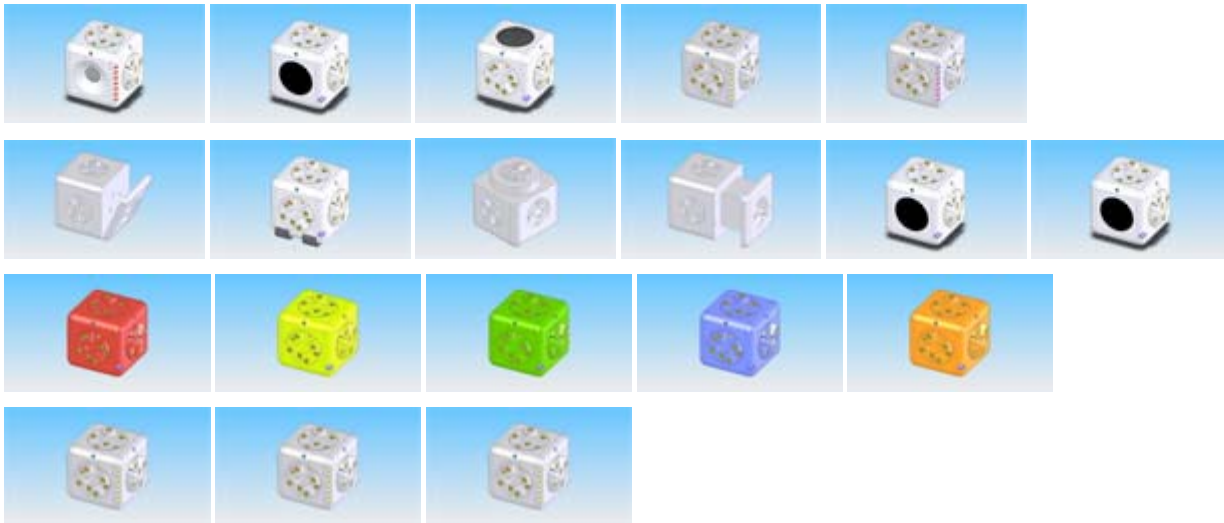
Figure 2. The roBlocks catalog. Top row (Sensors): Light, Sound, Touch, Motion, Distance. 2 nd row (Actuators): Hinge, Tread, Rotation, Extension, Siren, Flashlight. 3 rd row (Logic): Not, And, Or, Xor, Nand. 4 th row (Utility): Power, Comm, Passive.
