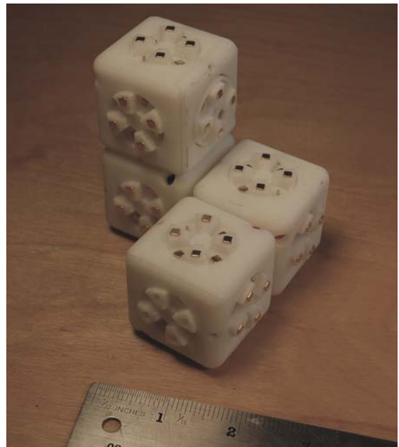
Figure 1. A simple roBlocks construction.
