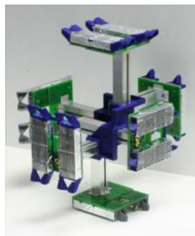
Fig. 8 Current prototype prismatic cube module showing core and six latch faces
