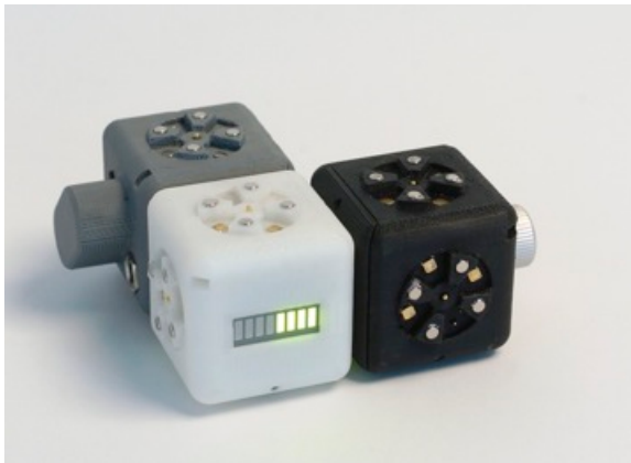
Figure 2. The simplest robot: a twist sensor block (the black block with a knob on the right) and a bar-graph action block. The gray block in back is a battery block.
