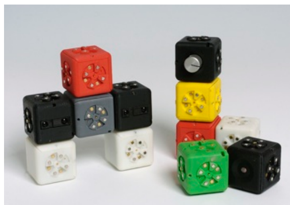
Figure 1. roBlocks is a heterogeneous modular robot construction kit. The white blocks are 'action' blocks, the black blocks are 'sensor' blocks, and the colored blocks are 'think' or
