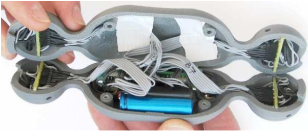
Figure 7: Strut shell open to show electronics inside.
