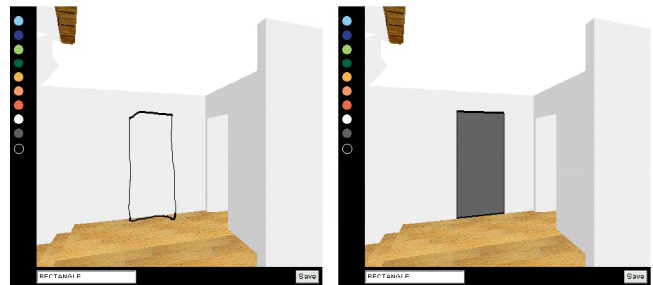
Figure 7. Adding a door on a wall. A rectangle drawn on a surface is recognized (echoed in the bottom left text field) and rectified (right).
