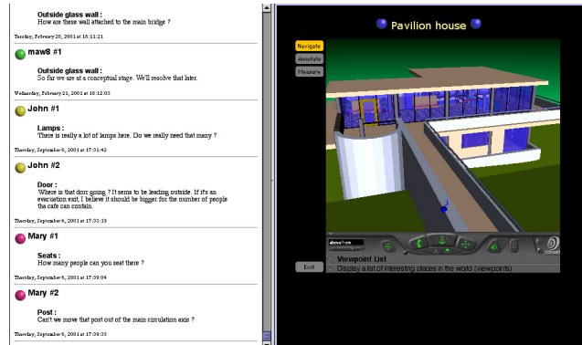
Figure 1. The Redliner interface: Left: Annotation window lists sorted comments. Right: The 3D interaction window includes four (mode) buttons and the CosmoPlayer navigation bar.
