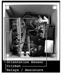
Figure 7. The main components inside a Block.
