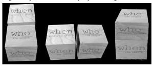
Figure 8. Using the Navigation Blocks to construct disjunctions and negations. Left: "or" query. Middle: "and" query. Right: "not" query.
