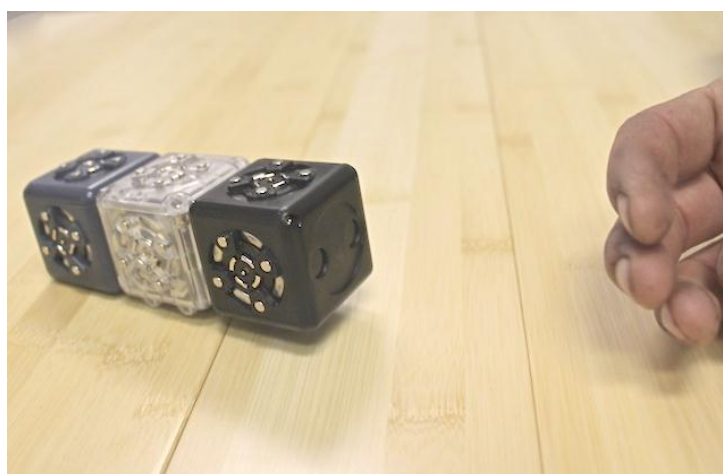
Figure 2. A three-Cubelet ‘follow-me’ robot made of a Distance and Drive Cubelet.
