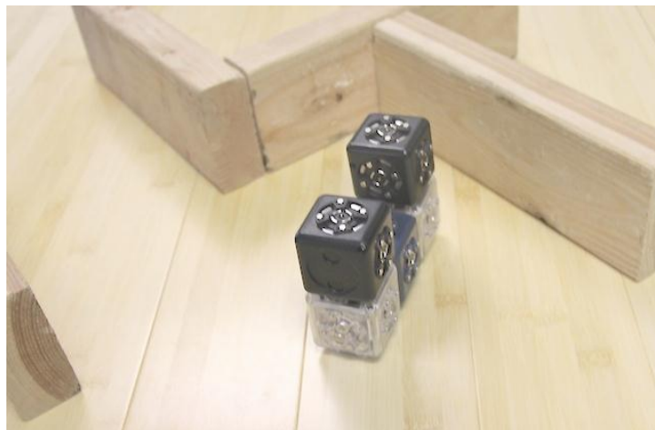
Figure 3. A Maze Solver: two Distance Cubelets, two Drive Cubelets and a Battery.
