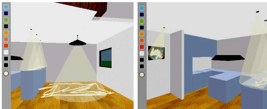
Figure 15. Light Pen system provides lighting fixture suggestions based on designer’s sketches.
