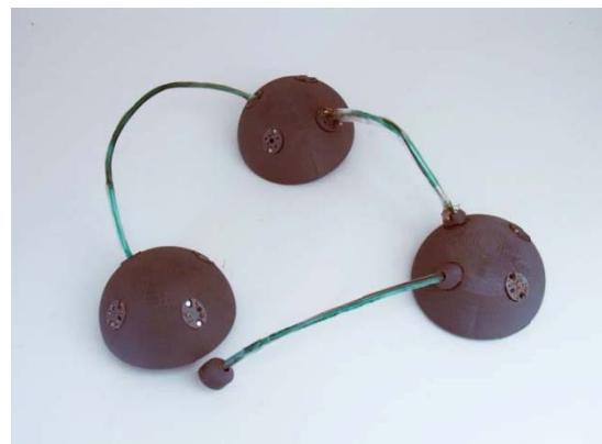
Figure 5. Edge connectors snap magnetically and connect electrically to the ports on the nodes. One node contains a battery and supplies power to the others.
