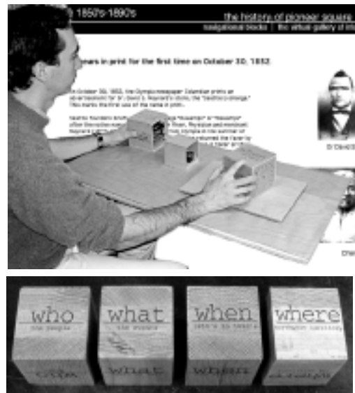
Figure 1a (top) A host Block (middle) receives information queries through infrared from the Block (right) on the active space and updates database display (background image). Figure 1b (bottom) Four Blocks support different query categories - who, what, when and where.
