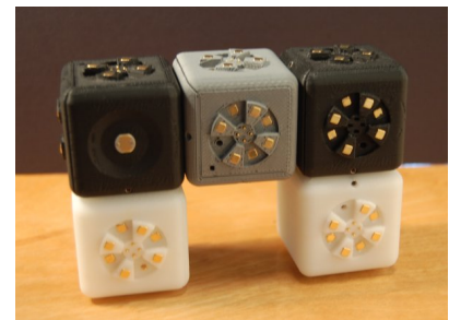
Figure 4: A mobile robot that steers away from light sources
