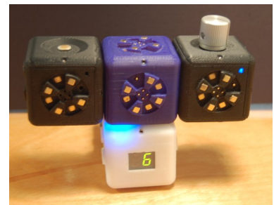
Figure 1: A little robot that operates based on the values of two connected sensor blocks
